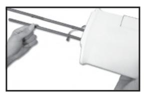
10. Insert the metal pipes to the main wing.
