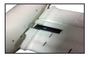
12. Connect the main wings to the fuselage and fix them by plastic clevis. Ensure that a sound of "click" to tighten the main wings to the fuselage.
