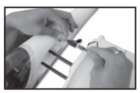
11. Put the metal pipes through the corresponding hole of the fuselage and connect the servo wires of the ailerons and flaps.
