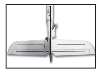
After connecting the clevises to the control horns view the vertical tail and rudder from directly above. The rudder should be 'in line' with the vertical tail when it's properly 'centered'. However, if the rudder is angled off to the right or left you can adjust the length/position of the pushrod/clevis so the surface is centered 'mechanically' while the trim lever on the transmitter is centered.
