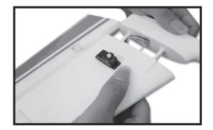
4. Install the rudder to the fuselage by screw.
