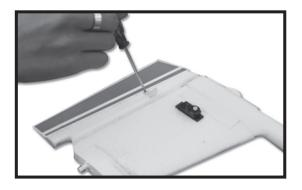
5. Install all the servo horn by screw.
