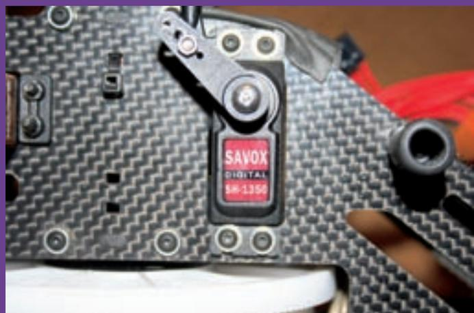
The Savox SH-1350 is a good all round servo that can be specified for a popular mid-size model like the T-Rex 500 for the CCPM and tail. See table for details
