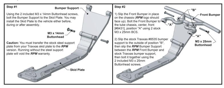
**Tip:** To simplify maintenance, any of the three pieces of the skid plate can be removed from the vehicle without removing the other parts. This allows faster access to the A-arm hinge pins, front bulkhead tie bar, tube chassis (center, front) and upper bumper support.
