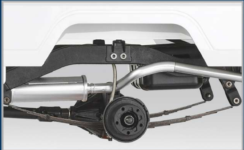
Rear Suspension: Leaf springs w/damper cylinder
