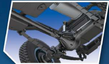
Rear suspension: Leaf spring w/damper cylinder
