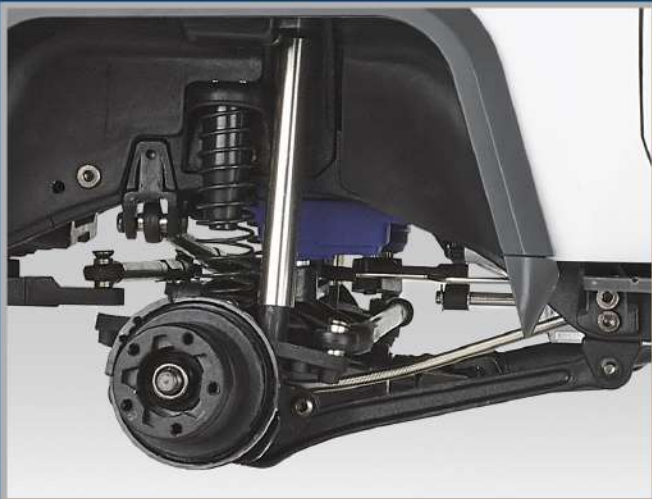
Front Suspension: 3-linkage suspension w/coil springs
