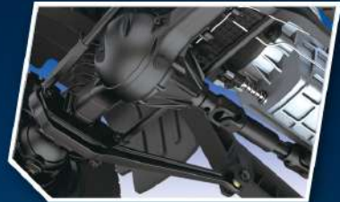
Rear suspension: Leaf spring w/damper cylinder
