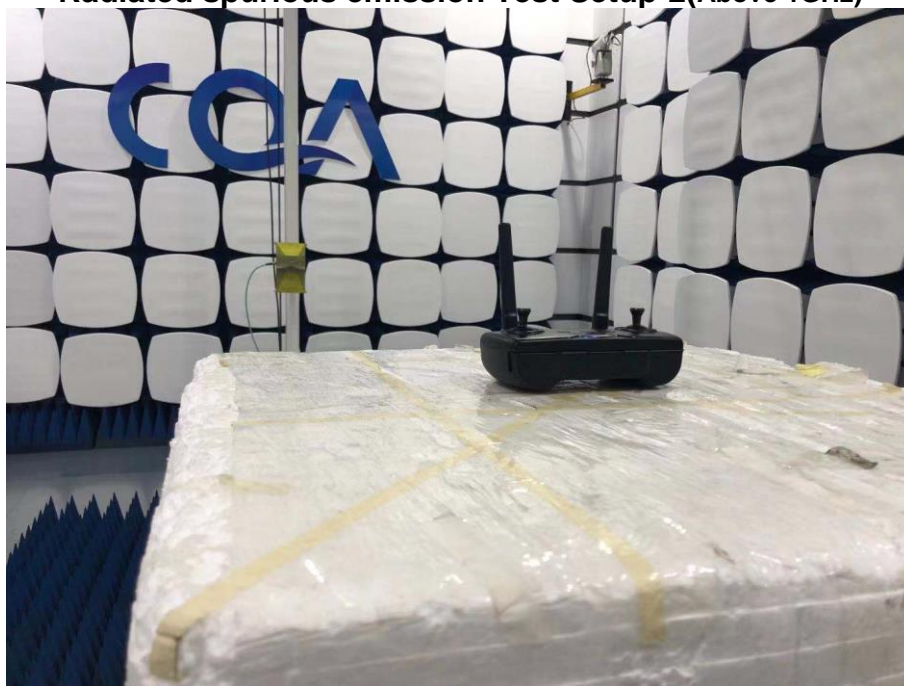
Radiated spurious emission Test Setup-2 (Above 1GHz)
