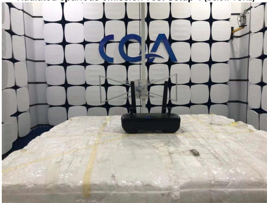
Radiated spurious emission Test Setup-1 (Below 1GHz)
