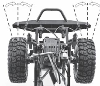
Gently pull the trigger to allow your car to run slowly. Meantime, tune the steering trim to allow the front wheels to be aligned.
