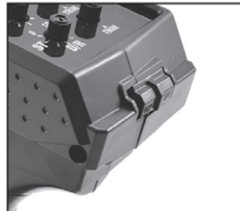
Switch on the power switch on the radio controller. Your car is bound with your radio controller automatically.
