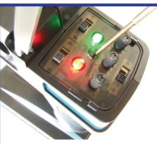
With the power on you can release the bind button once the green LED begins to flash to indicate the "Bind" process has initiated.
