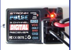
To 'Bind' the receiver to the transmitter the supplied Bind Plug should be installed channel 3/bind socket before power is applied. The red LED should begin to flash to indicate the 'Bind' process has begun, and go solid red once 'Bind' is complete. Now remove the 'Bind' plug and restart the power up procedure.
