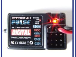
Unless a battery powered model using an ESC with BEC, a receiver pack should be plugged into the VCC socket via a suitable power switch, making sure to check for correct polarity.
