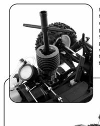
1. Before attempting to start the engine from cold,remove the glowplug with an 8mm nut driver prime the engine with fuel pull the pullstarter rapidly with your finger over the exhaust pipe outlet (IMPORTANT- only when cold!) until the fuel has travelled to the carb, and then a further 10-20 times to lube the engine.
