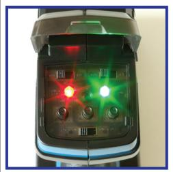
If the transmitter batteries are weak and the voltage drops below 9V DC, the green LED flashes to alert you to the possibility that range will be limited and control might be lost, so new batteries (or a recharge) are
