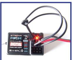
Once the 'Bind' process is complete, the throttle failsafe position can be set by pressing the button using the pointer provided.
