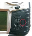
Press the "ENT" button and switch on transmitter (Tx), the Tx LCD screen flashing
