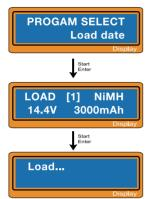
This program calls back the data that was stored at 'Save Data' program. To load the data, press **Start/Enter** key once to blink the data number field and select the number using **INC** or **DEC** key then press **Start/Enter** key for more than 3 seconds.
