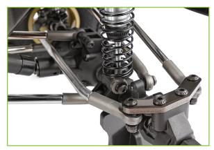
**BTA STEERING & ALUMINUM STEERING PLATES:** Behind-the-axle steering provides better approach angles, more clearance, and a cleaner look. Bolt-on aluminum steering plates allow for more adjustment, strength, and future modification for the user.
