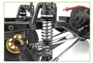
THREADED ALUMINUM SHOCK BODIES: Threaded aluminum and fluid-filled, these shocks keep the vehicle stable on the trail and retain oil even in the roughest terrain.
