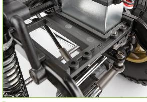
INTEGRATED SERVO WINCH MOUNT: Mounting a winch directly to the chassis is the strongest and most reliable spot on any trail rig. Positioned alongside the steering servo for overall chassis balance and weight distribution.
