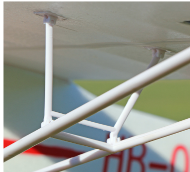
The jury struts are an important feature. Be careful to fit them the right way round!
