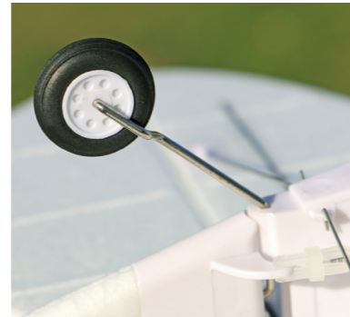
The tail wheel is overly long but I've since bent mine back for better effect.
