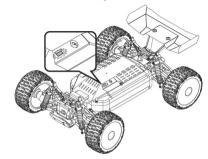
STEP 5: PRESS and HOLD the SW1 button on the transmitter and Power ON.
