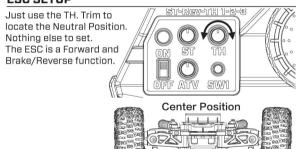
Maximum is 2S LiPo (7.4V) DO NOT EXCEED this voltage, otherwise will damage and void warranty.
