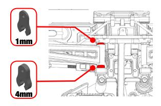
To change the Caster Angle, move the Upper Suspension Arm forward or backward using the different CASTER CLIPS sizes.
