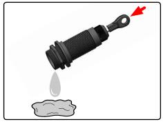
Drain the oil from the shock absorber.
