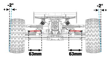
Adjust the angle by screwing the TURNBUCKLE.
