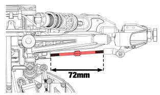
Adjust the angle by screwing the TURNBUCKLE.
