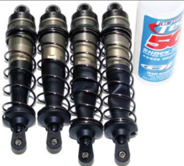
Left: Pre-assembled 16 mm big bore shocks with 4 mm shafts and over boots can take the punishment Right: Huge wheels and high speeds demand top spec servos. Fit the XP servo horns instead of the kit ones as they suit the XP spline pattern
