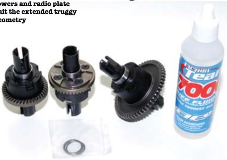
Above: Factory assembled differentials save a lot of time...
