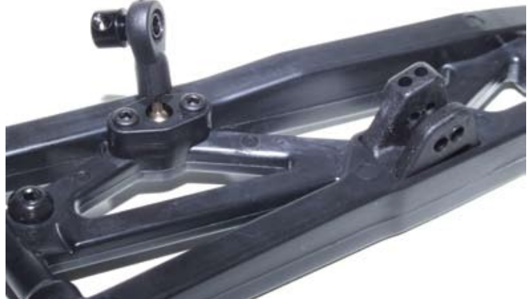
Below: Anti-roll bar linkage is adjustable from below, shock lower mount enhances angle and geometry. Droop screws included in all lower arms
