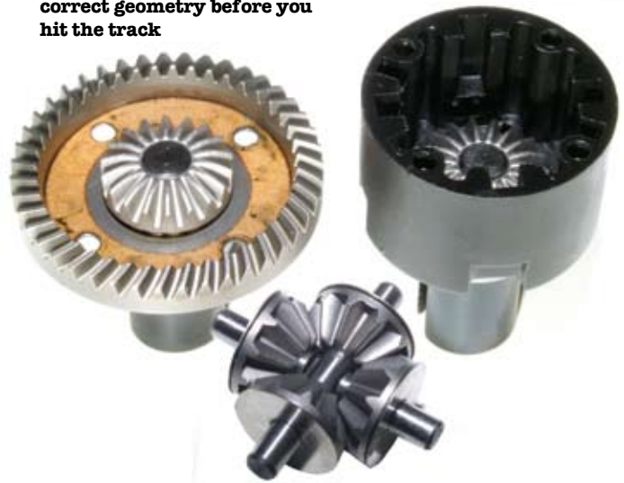
Above: ...but you still have to strip and lubricate each gear, pin and thrust washer before you run the truck
