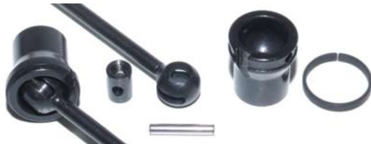
Above: Driveshafts have captive pins within bearing inners or spring clips. Nice with no grub screws
