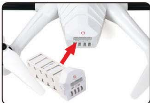
4.1.1 Install the fully charged battery DO NOT turn on the battery until later. *Please check the charger manual for charging instructions
