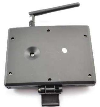
4. Attach the FPV screen to the handset mounted bracket by connecting the two halves together.
