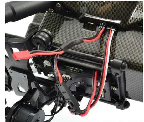
7. Install the video transmitter in a convenient location using the foam pad and cable ties provided to keep the wires tidy, then connect the red connector power lead from the video transmitter to the Y-power lead red connector.
