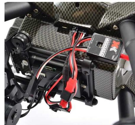
8. Connect the video lead to the X380-C camera USB connector, connect the other end to the black video transmitter connector. (The USB video lead is supplied with the FPV kit)
