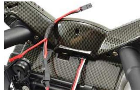
6. Connect the other side of the Y-power lead to the X380-C power port.
