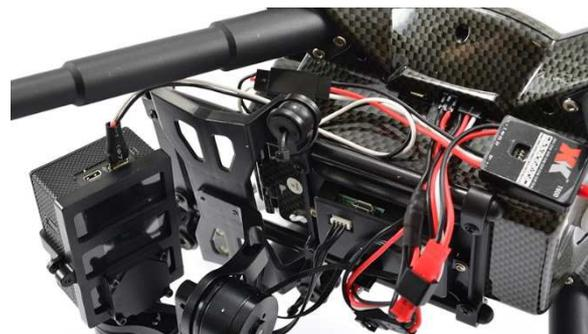
9. Turn on the X380-C, Camera and then FPV screen, the video will then be transmitting to the 4.3" FPV screen
