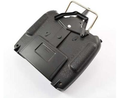
2. Place the front half of the screen holder on the front of the transmitter in-line with the rear holder and screw in place with the two thumb screws and nuts provided.
