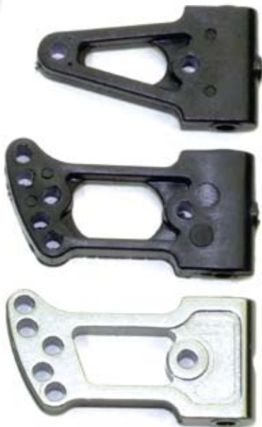
Above: RTR headstock (upper) compared to the race (middle) and alloy (lower) options
