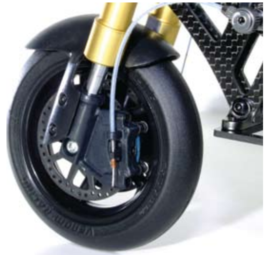
Above: Assembled front calliper with cable secured with clench collet. Remove the callipers and mudguard to swap front tyres
