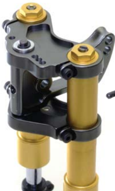
Above: Alloy triple clamps and headstock with ball bearing headraces make a solid front end. Note fork spring preload adjuster screws!
