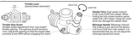
If the engine stalls on acceleration, begins to bog or slow down at full throttle, or if there is a reduction in exhaust smoke, then the engine is running too lean. Immediately turn the high speed mixture screw counterclockwise 1/4 of a turn and operate the car at medium speeds for 1 to 2 minutes to allow the engine to cool.
