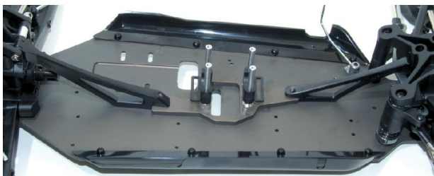
Sturdy chassis. The centre reinforcement connects the front and rear braces
