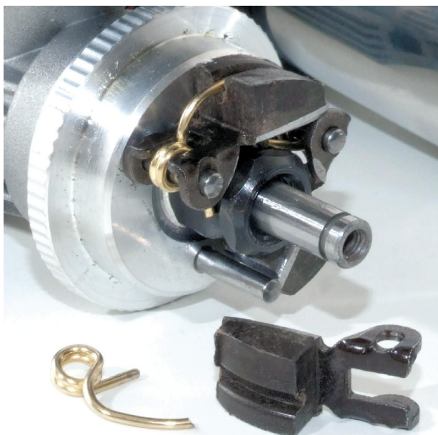
A unique lightweight clutch, fabricated shoe wearing a composite pad
