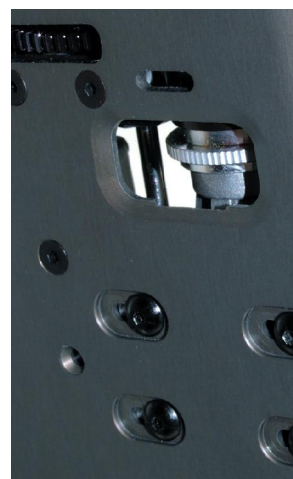
The chassis is chamfered to ease bump box access
