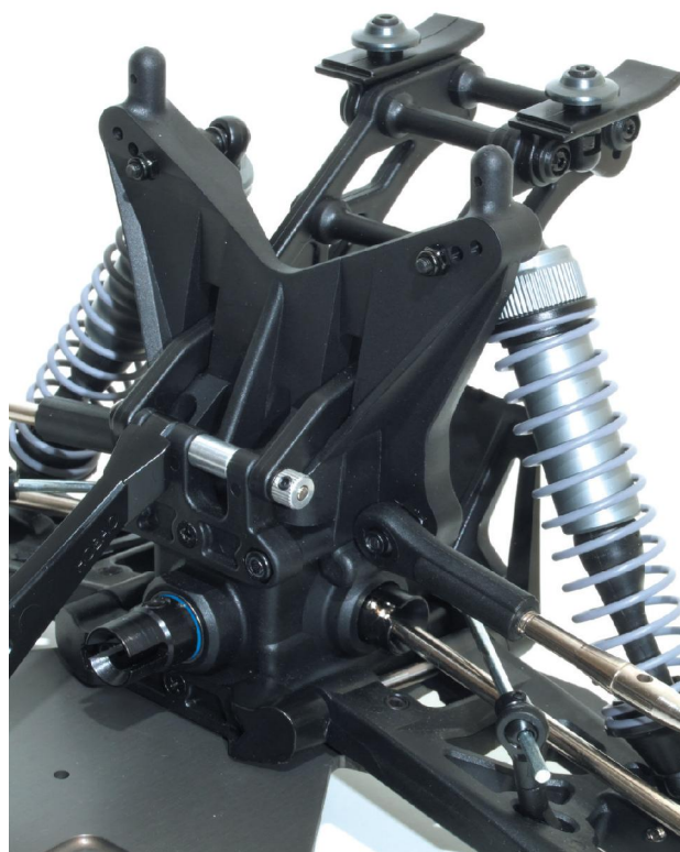
Diff cases, shock towers and braces combine for a rock solid assembly
