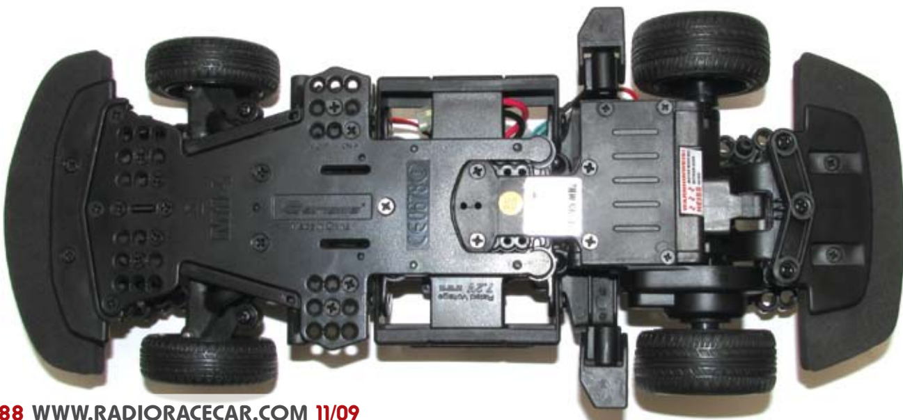
BELOW: Note the multiple body post locations and various sub assembly positions to suit different wheelbase versions
