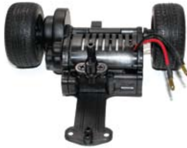
ABOVE: The floating rear pod takes its influences from 1/12th on road racing
