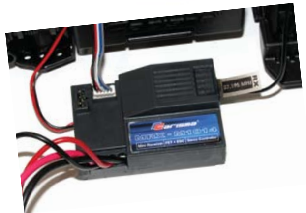
ABOVE: The 27 MHz receiver/ESC combo is future-proof, allowing the use of a standard 3-wire servo to replace the 5-wire unit fitted
