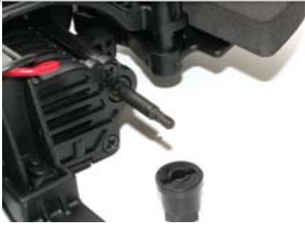
ABOVE: Pin drive plastic hexes ensure the rear wheels are fixed securely to the rear axle
