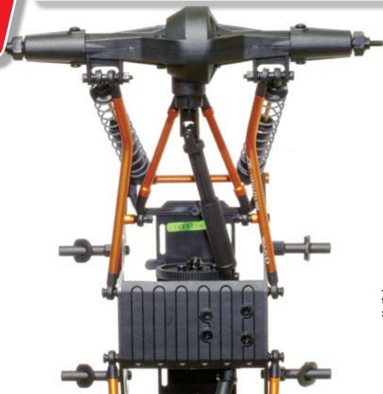
Above: Straight rear axle keeps the rear wheels parallel under load
