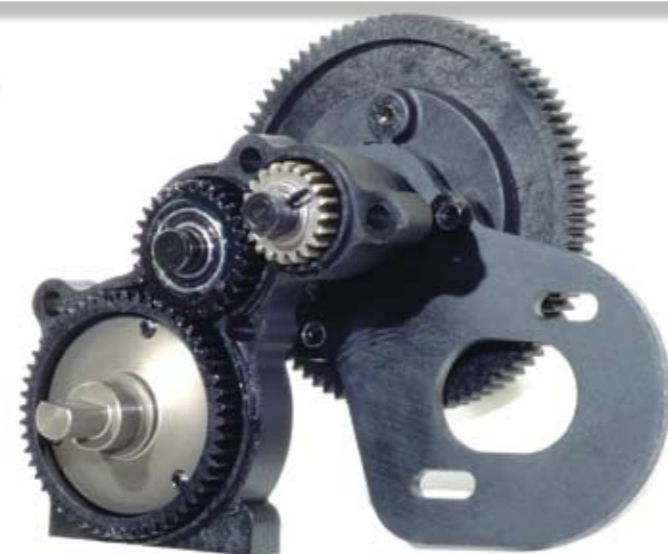
Above: Overall gearing ratio can be varied from 15:1 to 74:1 thanks to the 2.6:1 centre transmission getting it down in the first place
