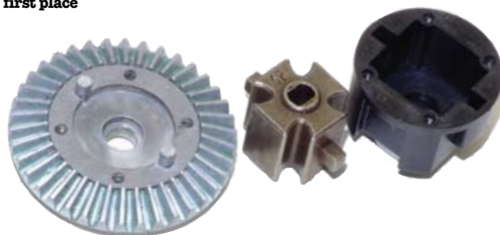
Above: Sintered diff lockers keep all four wheels working for you, permanently
