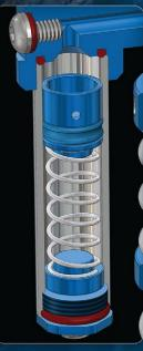
The **Ultra Reservoir Shocks** feature Dual Rate Springs and these shocks come with an extra collar so you can adjust exactly where the dual rate springs transitions to single rate, similar to full scale shocks!
