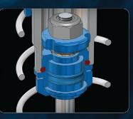
X-Ring seals are used for both the main shaft seal and the divider piston for the smoothest and lowest friction seal possible for these 9mm Bore Shocks.
