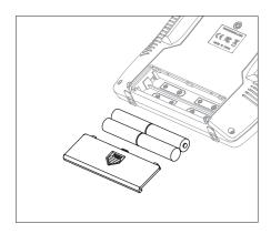
Remove the battery cover and install 4 AA batteries. Make sure the polarity of each corresponds with the diagram in the battery holder. Replace the battery cover.
