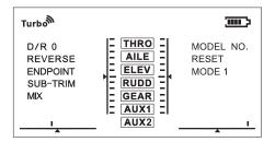
The EX7 comes with a digital LCD screen displaying a 3-level menu. Press Menu button to turn on/off background light of the screen. Following below instructions you are able to operate settings to EX7.
