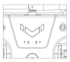
When the battery voltage drops below 4.3 volts, an alarm will sound and the voltage LEDs will flash.
