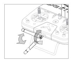
The EX6 comes with a retreatable antenna. When transporting, you can rotate it down at rear place to save space.
