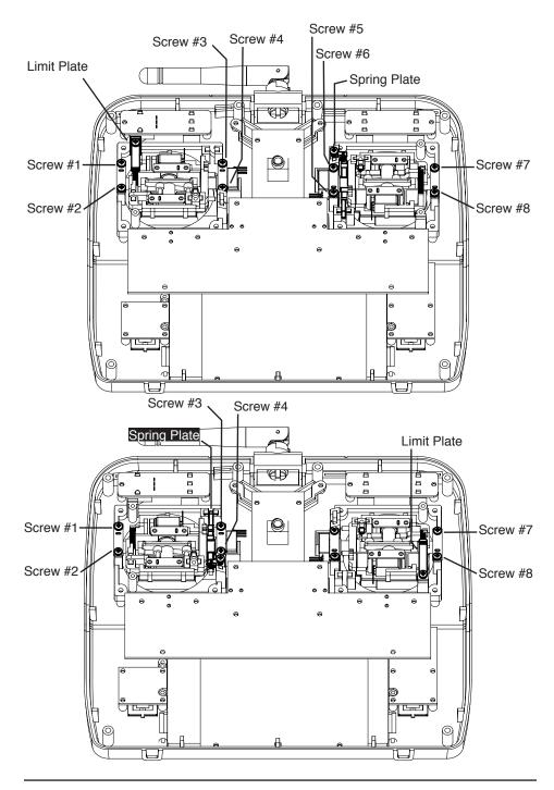
NOTICE: The mode 1/2 mechanical swich is using mode 1 swiched to mode 2 as example instruction. To switch from mode 2 to mode 1, just reverse the order of spring plate and limit plate.
