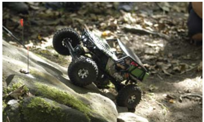
Above: Even in stock form the RTR Wraith coped well with the terrain, just needing a little weight adding to the front wheels to alter the bias and help pull itself up and over obstacles
