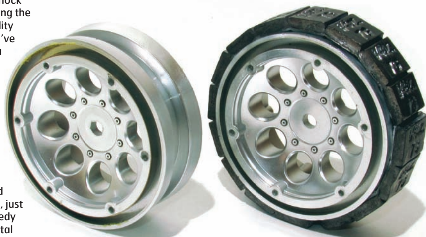
Above: The composite rear cage allows for extra lights to be fitted and adds to the rugged scale look Below: 5 oz of stick-on weight and venting the rims to allow the tyre carcass to deform makes a real difference on inclines and rocks
