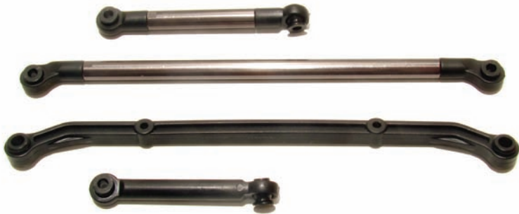
Above: Swapping out the plastic steering and drag links for alloy sharpened up the feel of the steering no end
