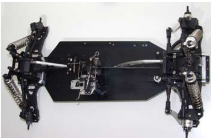
Above: Despite 4WD system the Punisher design makes for easy maintenance thanks to simple construction
