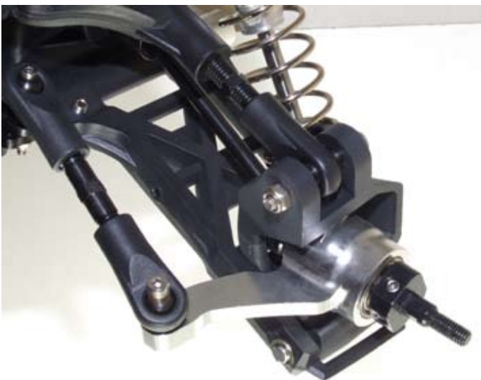
Above: The wheel drives have two grub screws holding it to the stub axle for extra security
