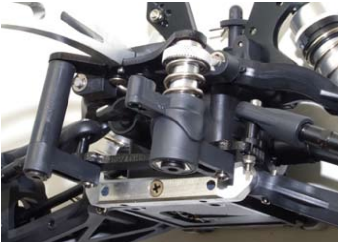
Above: Suspension pivot braces are substantial. Servo saver is overlapping to prevent dust ingress
