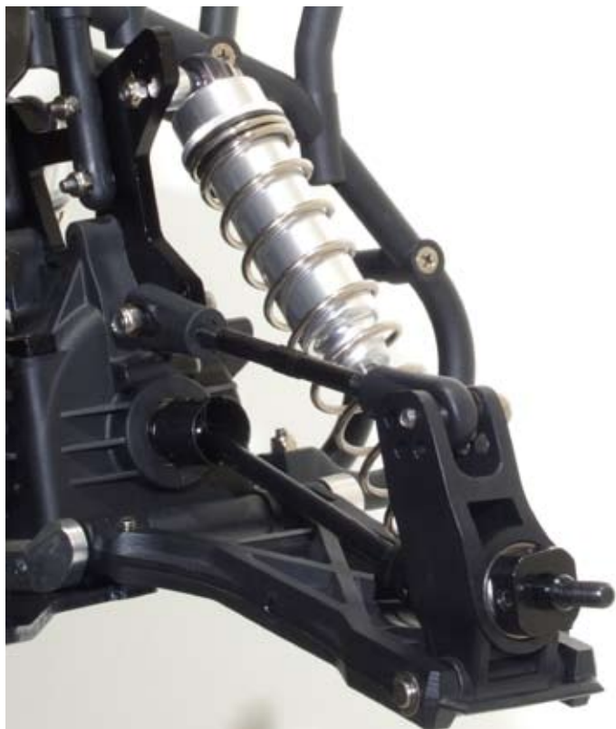
Above: Long travel suspension has droop to spare, note droop adjusting screw in lower arm
