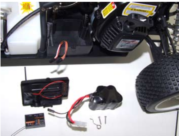
Above: Just add a large receiver battery to the radio box and you are away!
