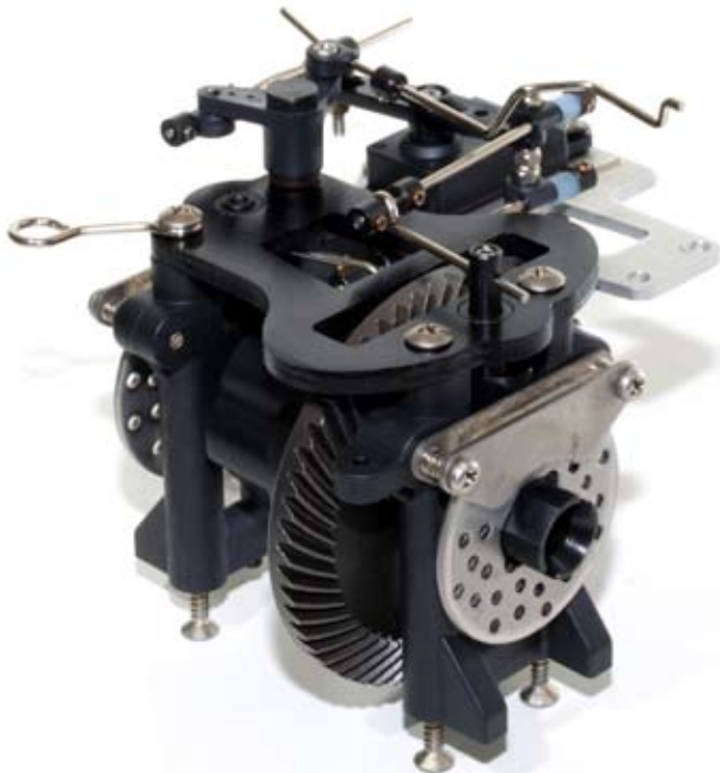
Above: Centre diff with brake assemblies means you can dial in front to rear bias perfectly
