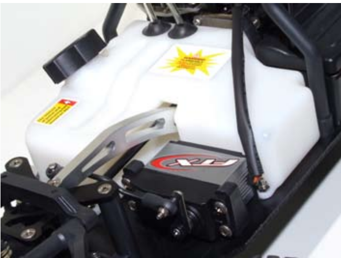
Above: Large steering servo has alloy cooling case, and surprising good performance for such a big unit!
