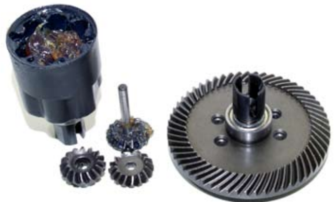
Above: Diffs arrive greased for running in but proper diff oils could be used to tune the driving style
