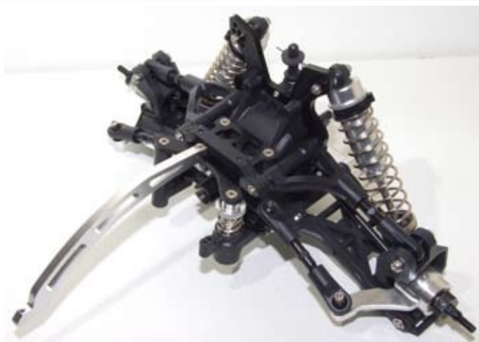
Above: The front drive and steering assembly, is supported by a large alloy chassis brace. Alloy hub carrier, shock tower, turnbuckles and large volume shock absorbers make this a high spec kit
