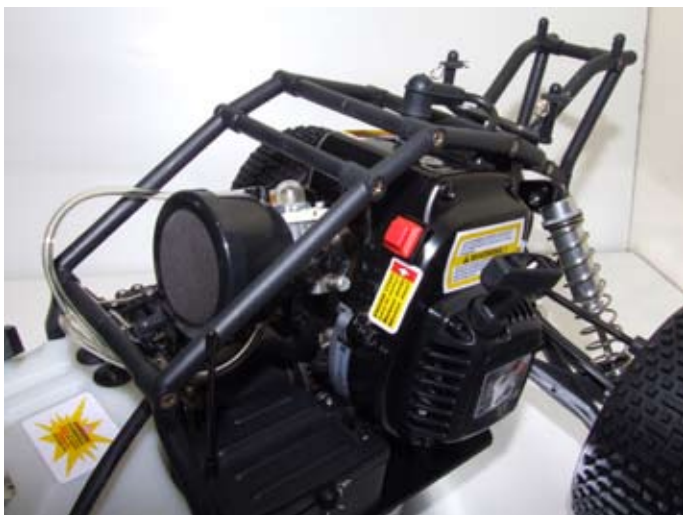
Above: The ignition kill switch is easy to reach, and is the only way to stop the engine unless you run out of fuel
