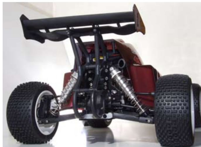
Above: Lots of roll centre adjustment with camber link positions inboard and outboard, plus shock angle choices means you can dial it in
