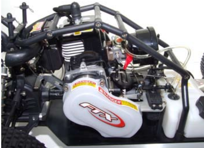
Above: Transmission has a guard to keep it covered, while engine is protected by a close fitting roll cage
