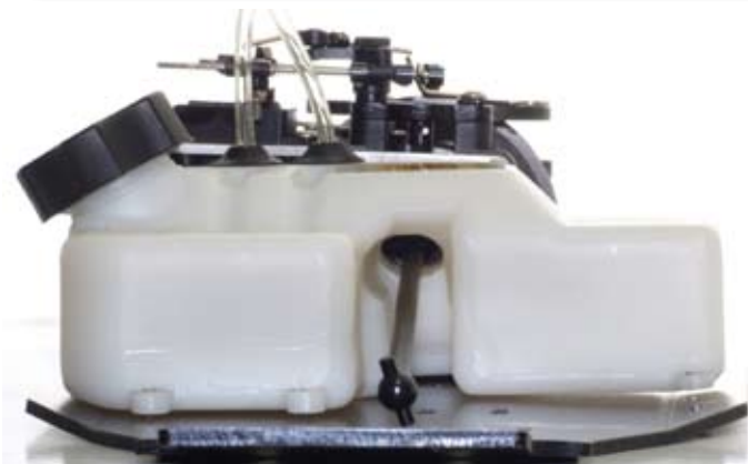
Above: How do you get drive forwards without splitting the fuel tank? Easy, go straight through!
