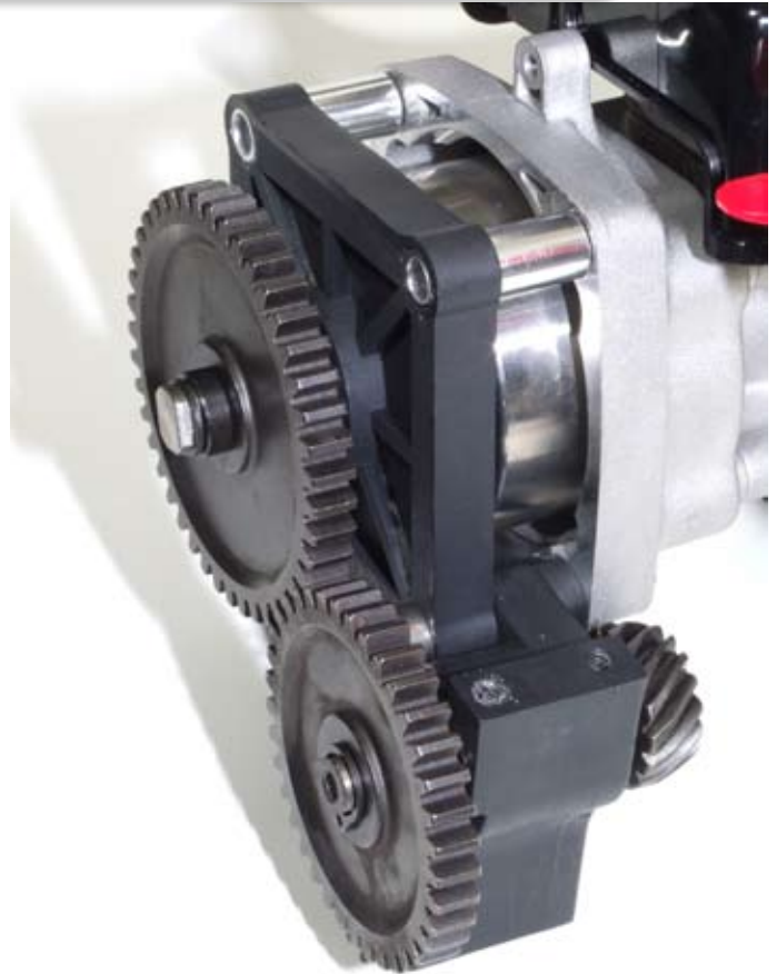
Above: All steel gears in the primary drive
