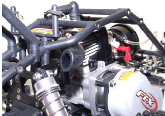
Above: Point the rubber exhaust exit rearwards to keep things clean under the body
