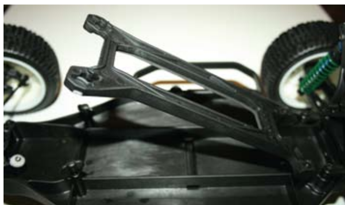
Below: The unique battery brace is simplicity in itself...
