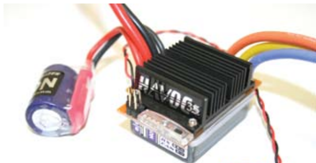
Above: Before I added the cooling fan, the Novak 'Havoc 3s' has all the usual family features and can now handle 3s LiPo too!
