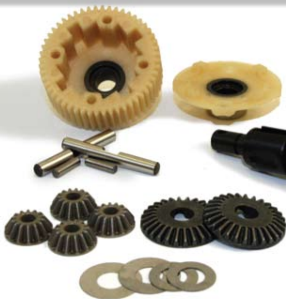
Above: Geared diff internals. Extra shims may be needed to get a good mesh
