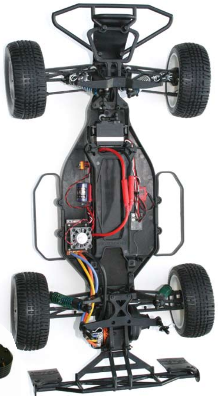
Above: Electrics installed with plenty of room. Check out the side nerf rails and bumper set-up!
