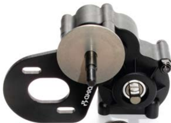
Right: With a well-adjusted slipper clutch, the entire drive-line is protected
