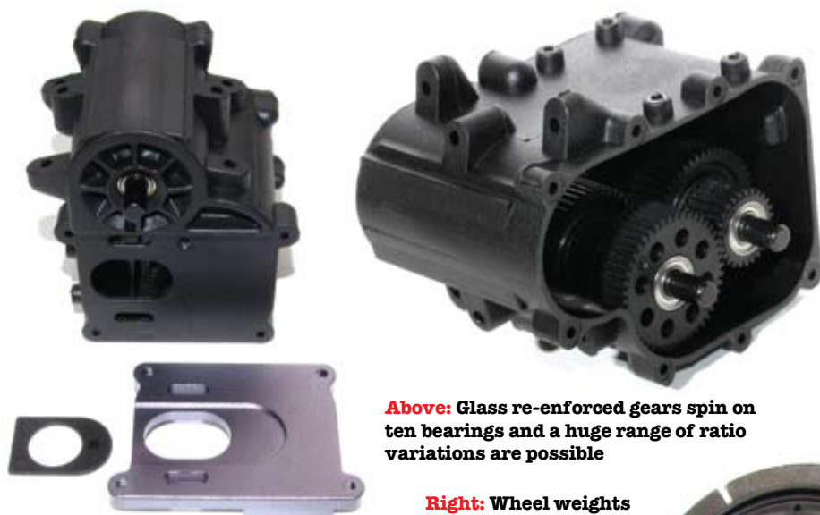
The transmission is a structural member and the backbone of the rig
