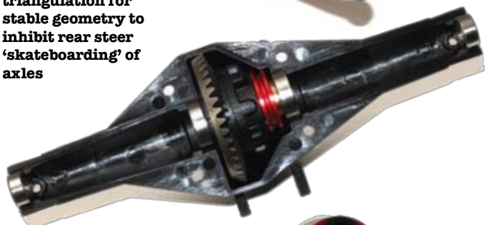
Locking diff mechanism installed in diff case, greased for smooth selector operation
