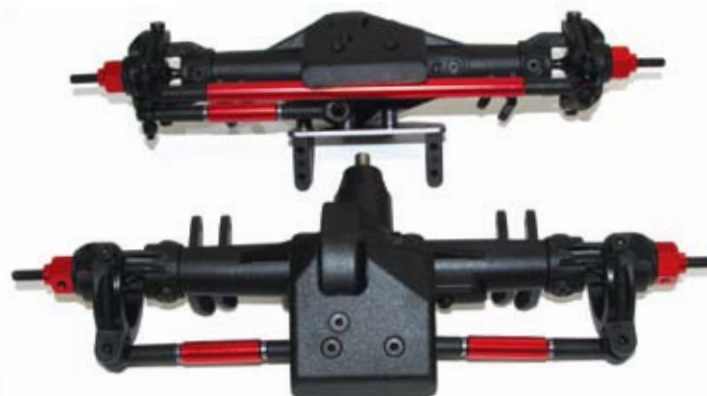
The skids protect the steering at the front but can get hung up at the rear in use
