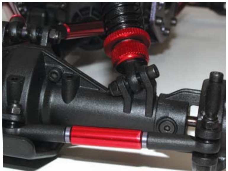
Angled lower shock mounts put the shocks at the perfect angle for smooth articulation
