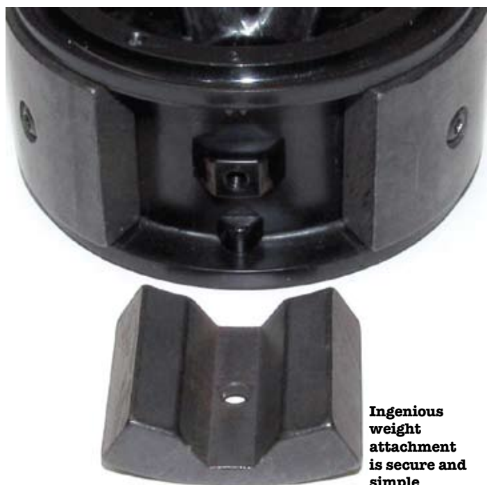
Beadlox system clamps the oval tyre bead between unique rim and clamp rings
