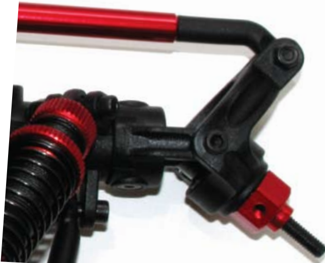
Amazing 40 degrees steering angle by design
