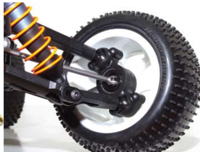
Below: Superb kit tyres. CV joint captures pivot pin in bearing. PBS is super smooth and slop free
