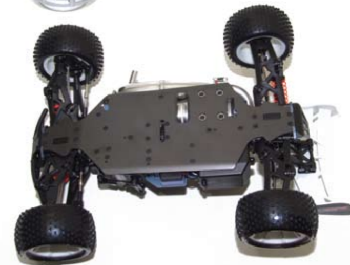
Below: Flush hard anodised alloy chassis has diff cases, spur gear, fly wheel and pull start recesses to get everything as low as possible
