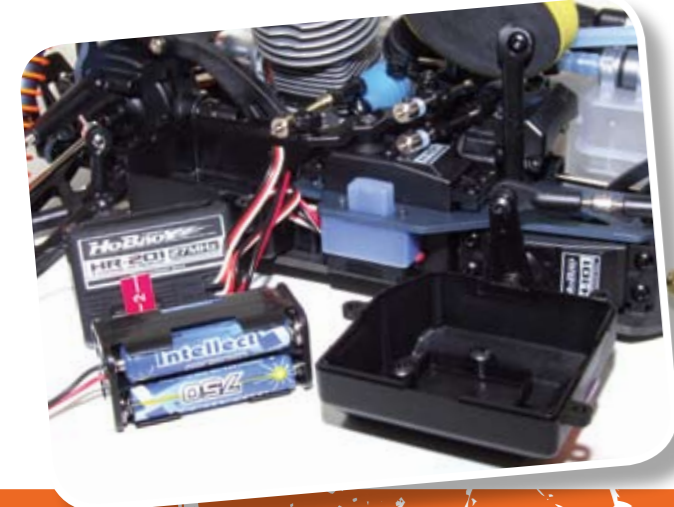
Below: Radio box has room for full size receiver and AAA battery pack. Note transponder mount in lid, rubber covered switch
