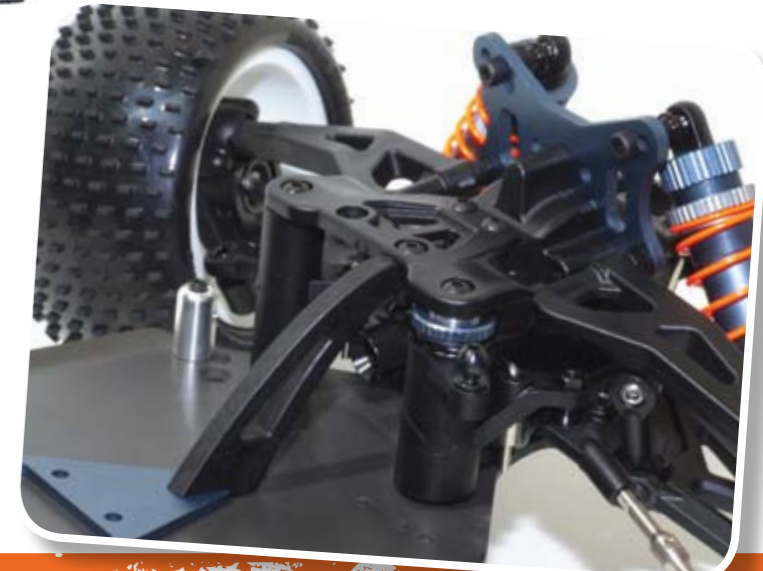
Below: Twin post steering, easy finger access servo saver adjuster nut, additional alloy chassis plate and diff case braces
