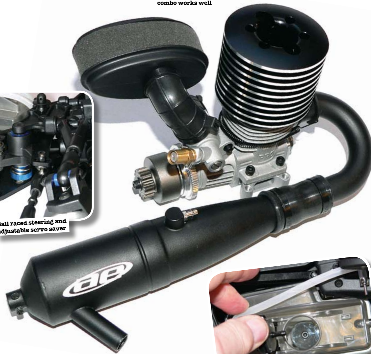
Pro 28 engine and AE 'outlaw' two chamber pipe combo works well
