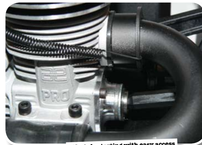
F1-style starting with easy access for hand held starter hex key
