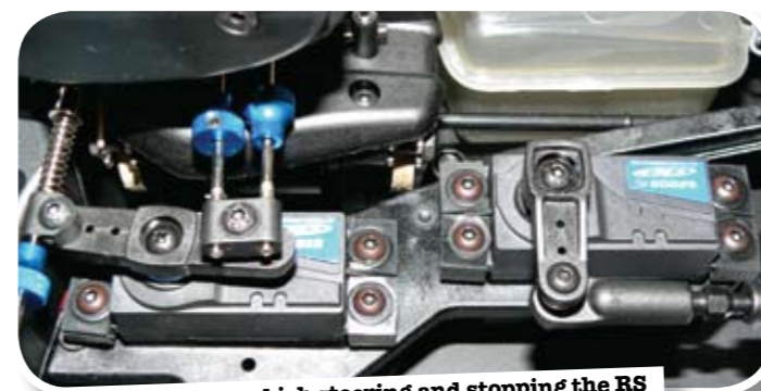
AE servos do good job steering and stopping the RS
