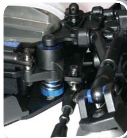
Ball raced steering and adjustable servo saver
