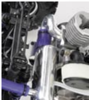
The alloy exhaust system uses a rubber extension to direct the gases away
