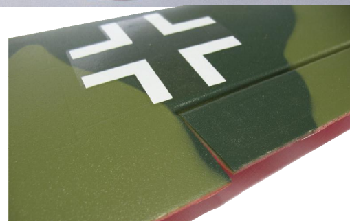
The neutral position for the ailerons offering, effectively, washout
