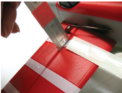
Feeding the transfers into the hinge apertures using a blunt instrument like the end of a steel rule
