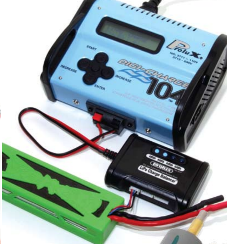
Above: Flexible Prolux charger and optional balance interface for safe LiPo balance charging up to 4 amps Right: Simply efficient, no brushes, no hassles
