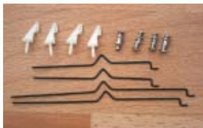
Hardware pack uses neat micro control horns and short wire linkages. Clamp connectors were not used on review model
