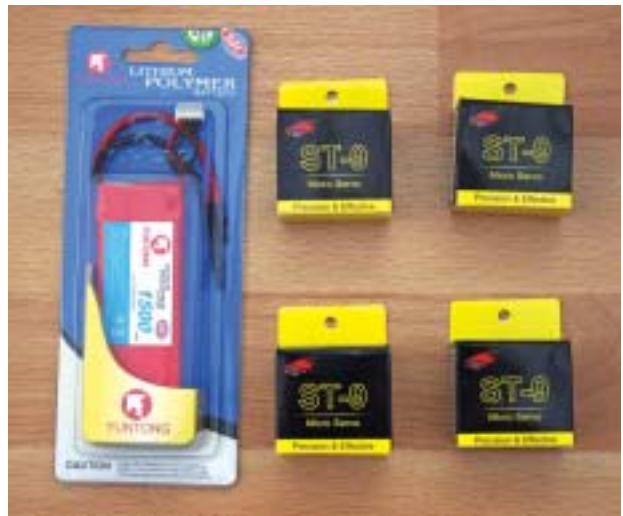
CML now distribute suitable servos and LiPo batteries. The 1500 3S pack is 25C (47.5 A) rated!
