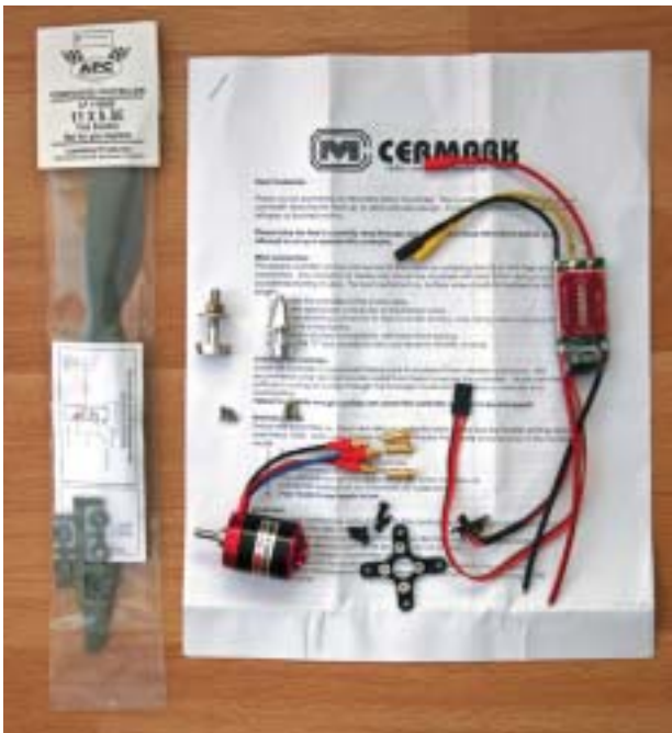
The CML motor pack contains an APC 11" x 5.5" E-prop, adaptors, motor, mount connectors and 30 A ESC
