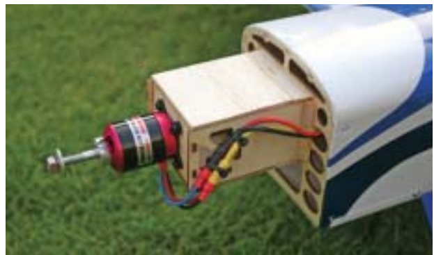
Engine box follows I/C pattern and is built up from ply and balsa. Unit slides into laser-cut slots in fuselage
