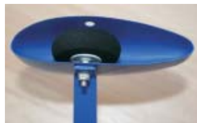
Vac formed spat covers 30 mm lightweight foam wheel
