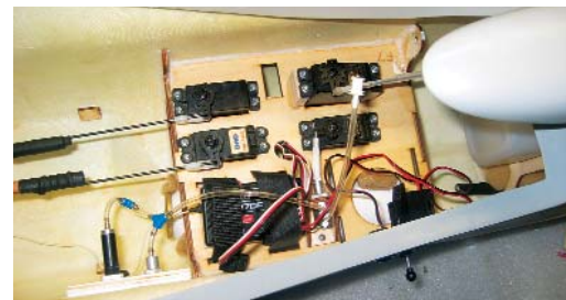
The servo tray holds the servos for the rudder (upper left), throttle (upper right), elevator (middle left), and retract valve (middle right) as well as the receiver and the retract air control valve. The pressure gage and air fill connector are located behind the servo tray.
