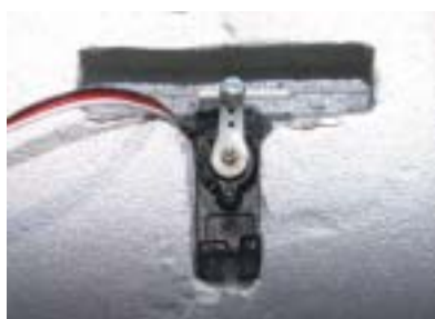
The aileron servo in place – a couple of dabs of hot glue do the trick
