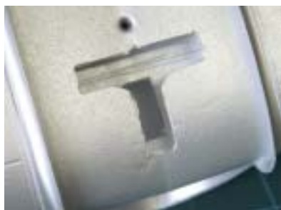
A servo slot needs to be cut into the lower wing panel
