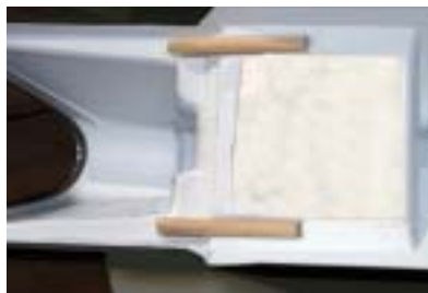
The dowel ends were rounded off to help the cockpit cover slide into place
