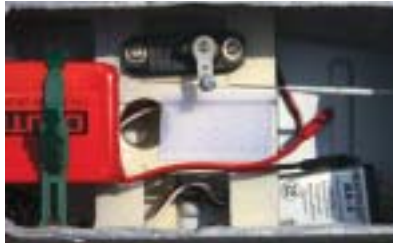
Placement of the electrics and the elevator servo
