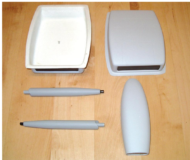
Moulded radiators and oil cooler with plug-in cannon shaped from balsa
