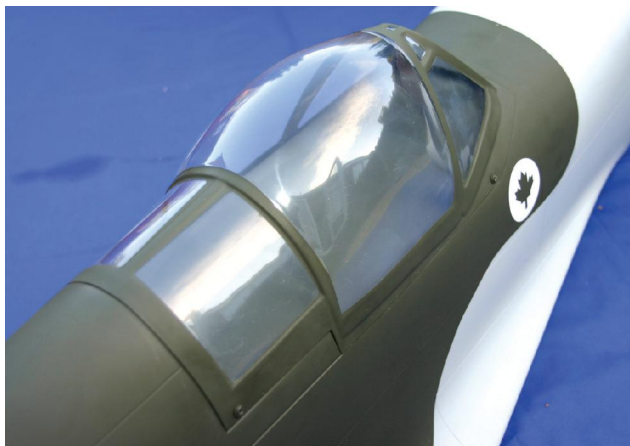
Super cockpit and framing attached by small screws
