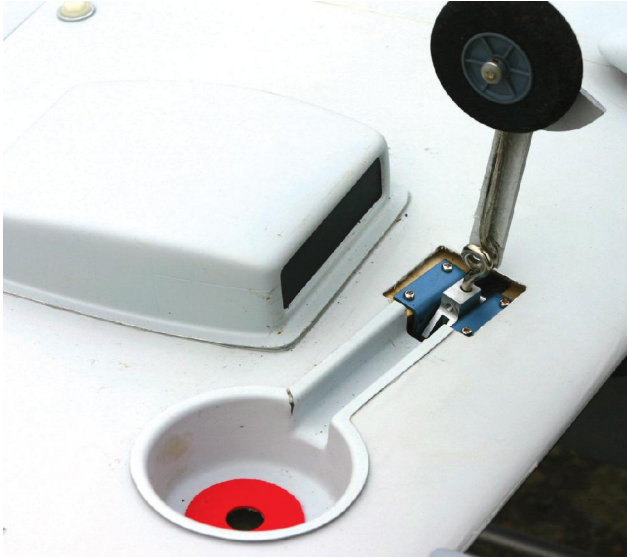
Collet relief hole in wheel well, and note the front shape of the radiator moulding
