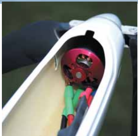
That light but powerful outrunner fitted to the Overlander speed controller
