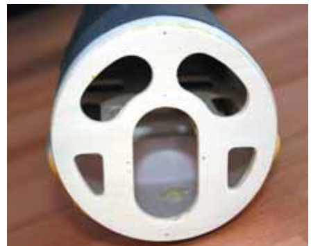
Lite-ply bulkhead is pre-drilled to suit the MPJ gearbox. Blanking piece can be glued in place to fit an outrunner
