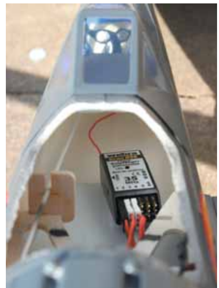
Synthesised receiver sits beneath cockpit, well clear of ESC and motor noise
