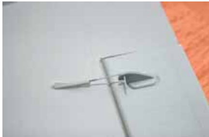
Ailerons are hinged using foam. Horn, snake and solid wire inner are ready fitted. Note panel lines
