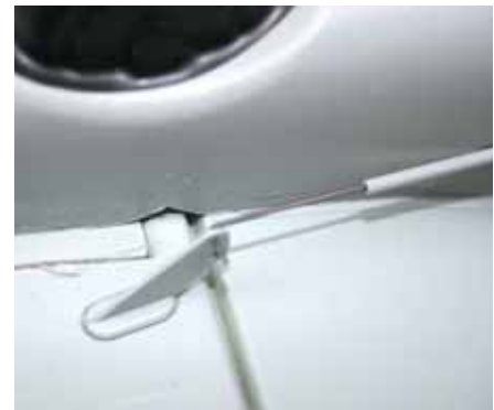
Tail is pre-fitted with horn and pushrod connected. Semi-recessed tailwheel is moulded in
