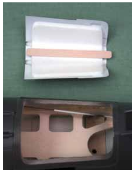
Neat clip on hatch provides access to battery and radio bay
