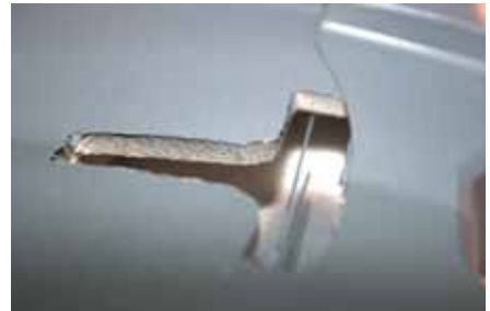
Aileron servo opening and snake wires. Detail of foam with hard skin clearly visible here
