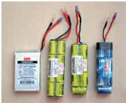
Packs used for test included 7 and 8-cell AR and a 2S LiPo
