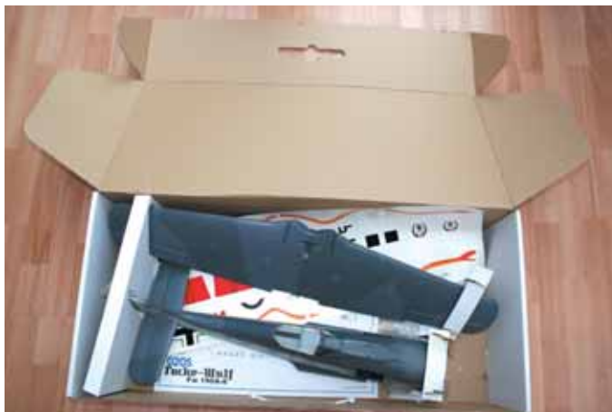
Open the box to reveal wing and fuselage complete, apart from decals, motor and radio gear
