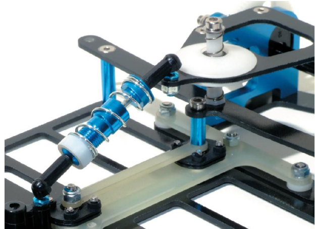
The rear shock. Note tweak screws not in 'T' Bar yet
